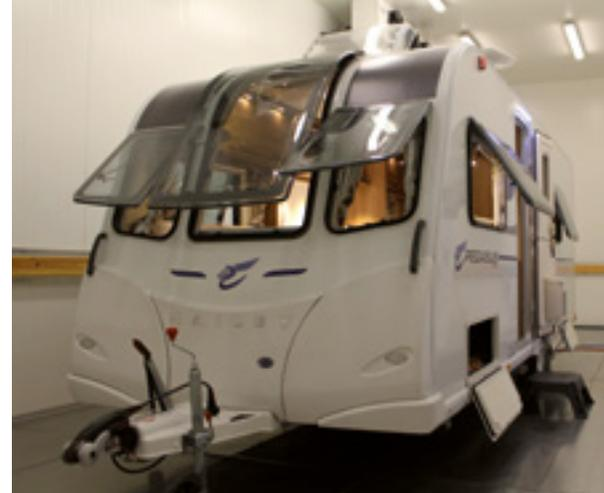
To meet this challenge, our designers created something truly ground-breaking. A patented aluminium external framework clamps the bodyshell panels together to create a shell that is so much stronger than anything that has gone before. Fewer external joints and fixing points make this shell more weather proof, while significantly thicker panels provide better insulation to keep you warm in the winter and cool in the summer.
