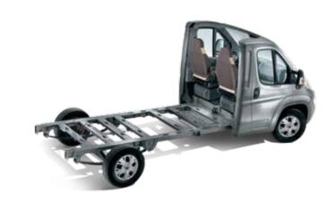
**Fiat Ducato** 2.3-I-Multijet **Basic engine** Engine power kw (BHP) 96 (130) Technically permissible maximum laden weight (kg) 3,495 Possible load capacity (optional, kg) 3.850 Trailer load 12 % braked/unbraked (kg) 2,000/750 215/70 R 15 C Water supply incl. boiler / wastewater tank (I) 122 (20) / 92 Battery / charger (Ah/A) 95/18
